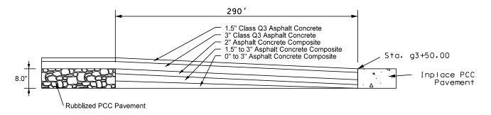
Ends of transition should start and stop at a joint in the PCC Pavement. Transition length may vary from what is shown above due to these joint locations.
