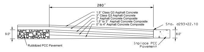
End of transitions should start and stop at a joint in the PCC Pavement.
