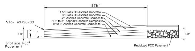
End of transitions should start and stop at a joint in the PCC Pavement. Transition lengths may vary from what is shown above due to these joint locations.
