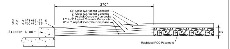
End of transition should stop at a joint in the PCC Pavement.
