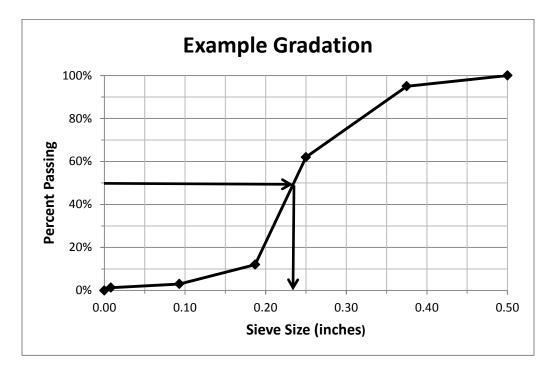
For the given gradation, the median particle size is determined to be  $\underline{0.23}$  inches.
