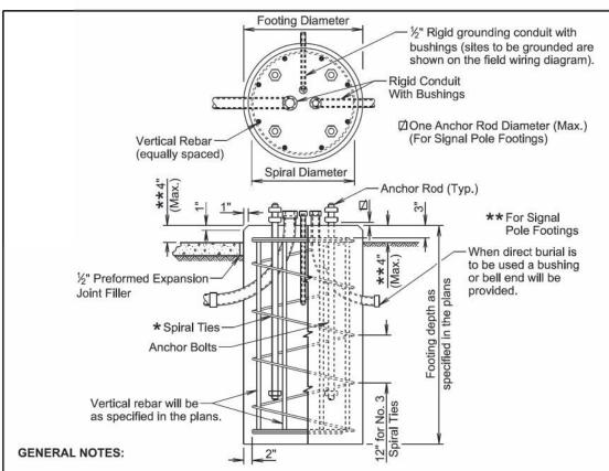
\* Circular ties may be used in lieu of the spiral ties. The No. 3 ties will be spaced 12 inches apart except for the top two which will be spaced 6 inches apart. The ties will be lapped 18 inches and the laps will be staggered around the cage.
