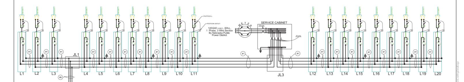
LUMINARE EXTENSION CIRCUIT NOTE: HOT LEG SHALL BE FUSED AT POLE BASE WITH A 10A FUSE
