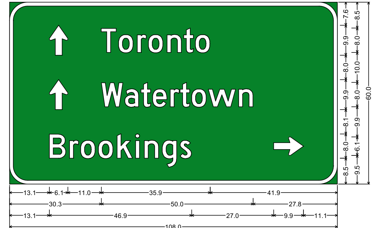
6.0" Radius, 1.3" Border, White on Green; Standard Arrow 2.25 9.9" X 6.1" 90°; "Toronto", D 2K; Standard Arrow 2.25 9.9" X 6.1" 90°; "Watertown", D 2K; "Brookings", D 2K; Standard Arrow 2.25 9.9" X 6.1" 0°;
