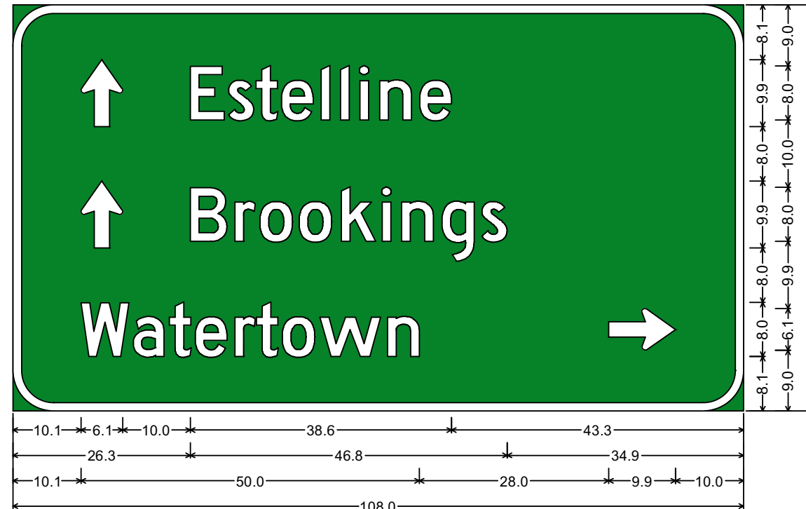
6.0" Radius, 1.3" Border, White on Green; Standard Arrow 2.25 9.9" X 6.1" 90°; "Estelline", D 2K; Standard Arrow 2.25 9.9" X 6.1" 90°; "Brookings", D 2K; "Watertown", D 2K; Standard Arrow 2.25 9.9" X 6.1" 0°;
