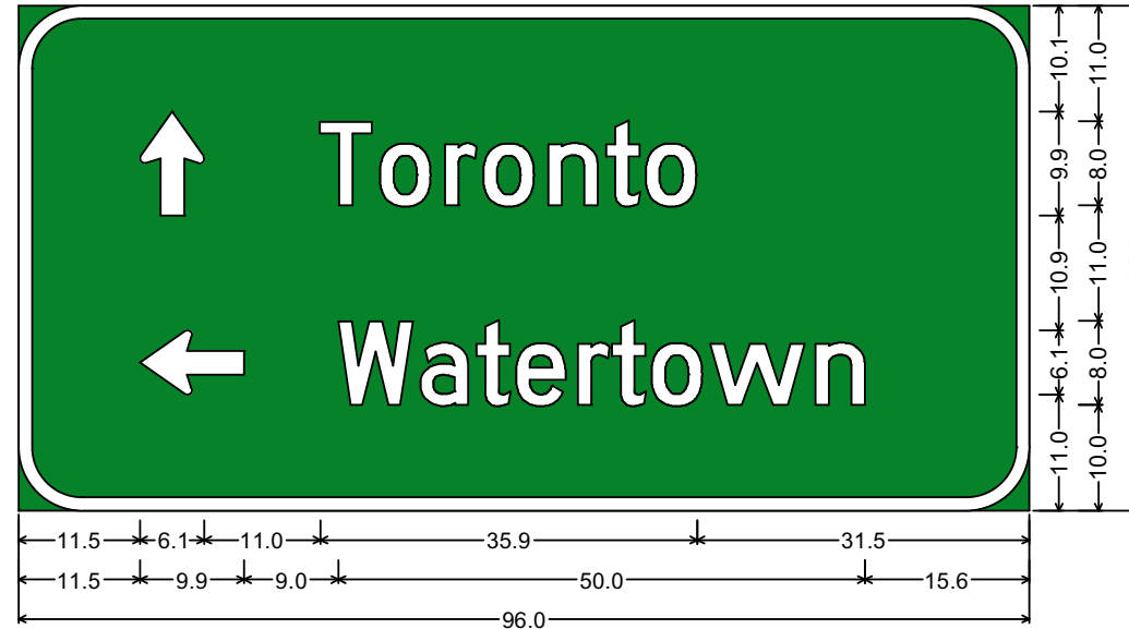
6.0" Radius, 1.3" Border, White on Green; Standard Arrow 2.25 9.9" X 6.1" 90°; "Toronto", D 2K; Standard Arrow 2.25 9.9" X 6.1" 180°; "Watertown", D 2K;
