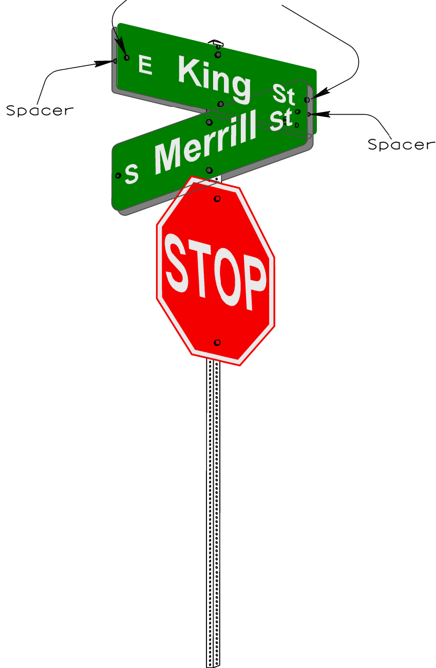
STOP SIGN WITH STREET SIGNS (TYPICAL ASSEMBLY)
