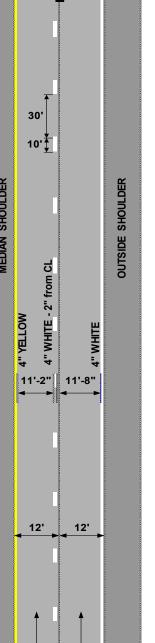
Typical pavement marking as shown on this sheet will be applied throughout the entire length of divided roadway.
