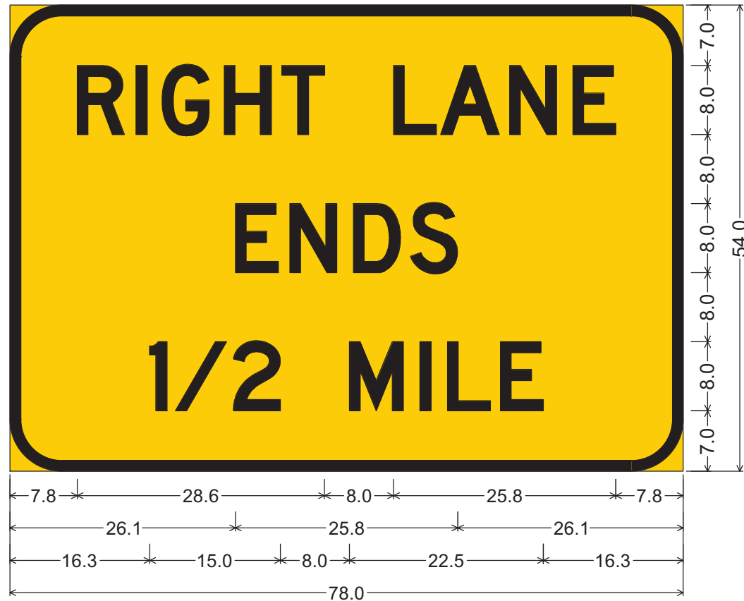
6.0" Radius, 1.3" Border, Black on Yellow; "RIGHT LANE", D 2K; "ENDS", D 2K; "1/2 MILE", D 2K;
