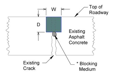
\* Inert compressible material required for cracks 3/8" or more in width. The backer rod will be a nonmoisture absorbing, resilient material approximately 25 percent larger in diameter than the width of the joint to be sealed. The backer rod will be compatible with the sealant and no bond or reaction will occur between the rod and the sealant.
