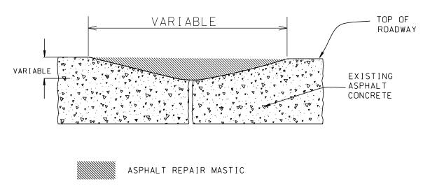
\* MULTIPLE APPLICATIONS OF THE ASPHALT REPAIR MASTIC MAY BE REQUIRED TO ADEQUATELY LEVEL THE JOINT AS DIRECTED BY THE ENGINEER.
