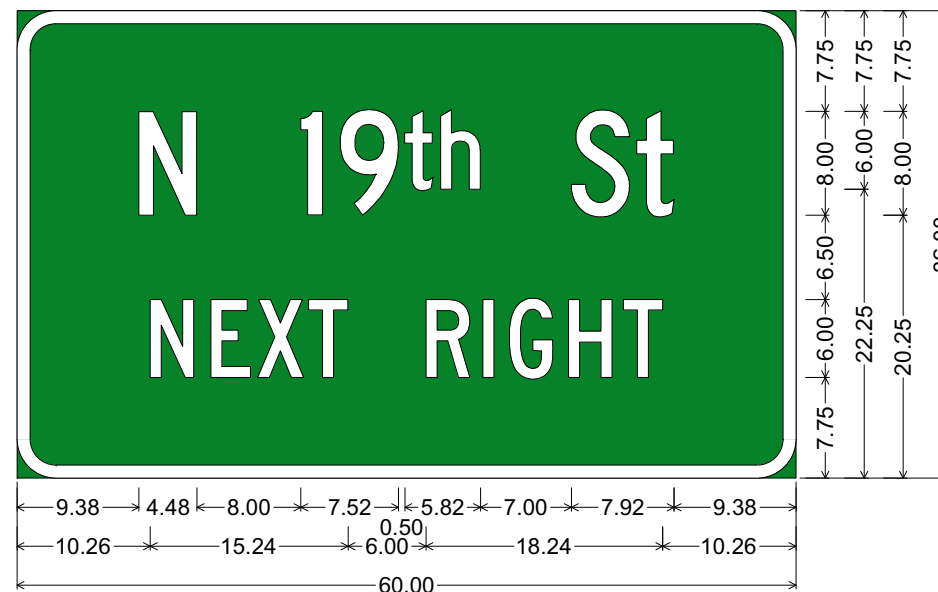
3.00" Radius, 1.00" Border, White on Green; "N", C 2K; "19th", C 2K; "St", C 2K; "NEXT RIGHT", C 2K;
