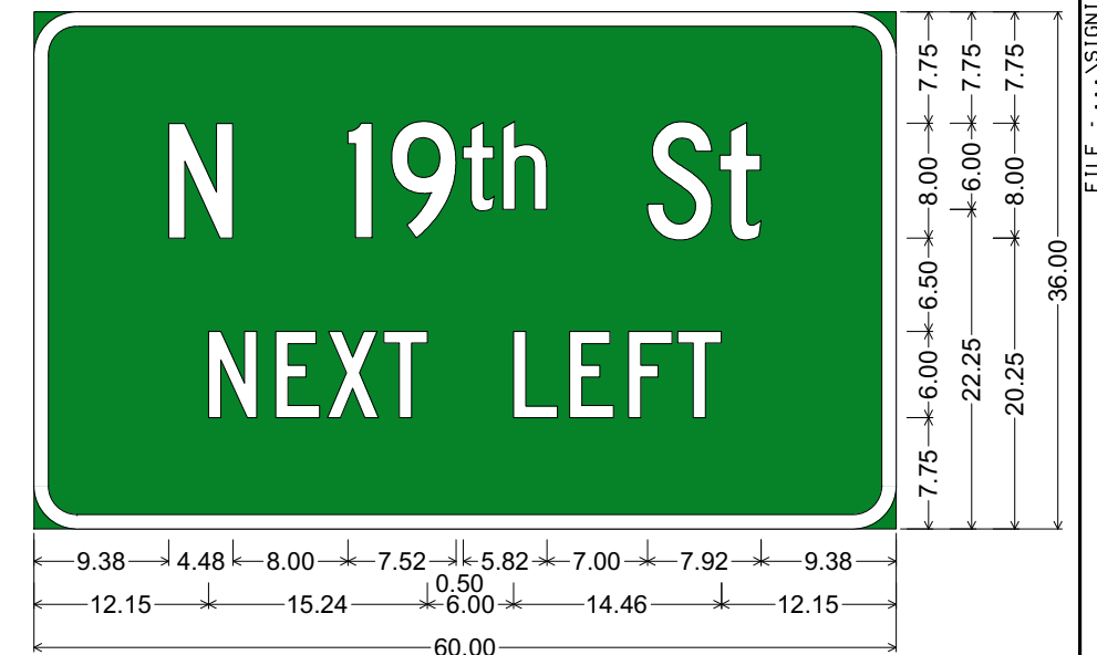
3.00" Radius, 1.00" Border, White on Green; "N", C 2K; "19th", C 2K; "St", C 2K; "NEXT LEFT", C 2K;
