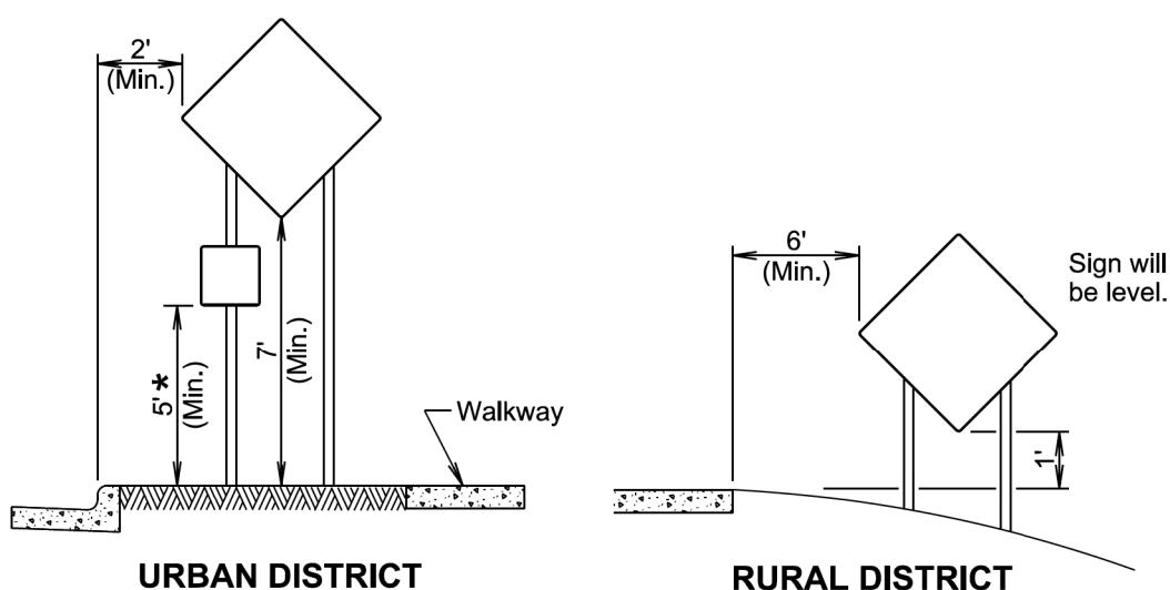
\* If the bottom of supplemental plate is mounted lower than 7 feet above a pedestrian walkway, the supplemental plate should not project more than 4" into the pedestrian facility.
