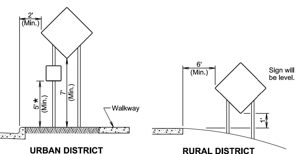
\* If the bottom of supplemental plate is mounted lower than 7 feet above a pedestrian walkway, the supplemental plate should not project more than 4" into the pedestrian facility.
