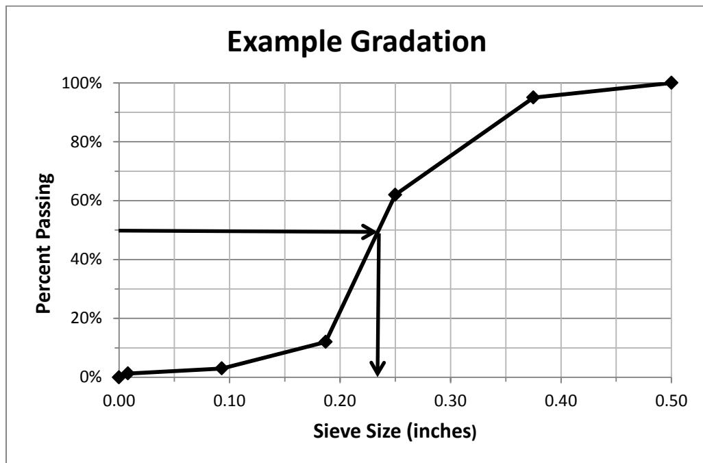
For the given gradation, the median particle size is determined to be 0.23 inches.
