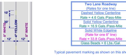
Typical pavement marking as shown on this sheet shall be applied throughout the entire length of undivided roadway.
