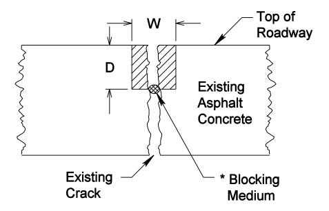
\* Inert compressable material required for cracks 3/8" or more in width. The backer rod shall be a nonmoisture absorbing, resilient material approximately 25 percent larger in diameter than the width of the joint to be sealed. The backer rod shall be compatible with the sealant and no bond or reaction shall occur between the rod and the sealant.
