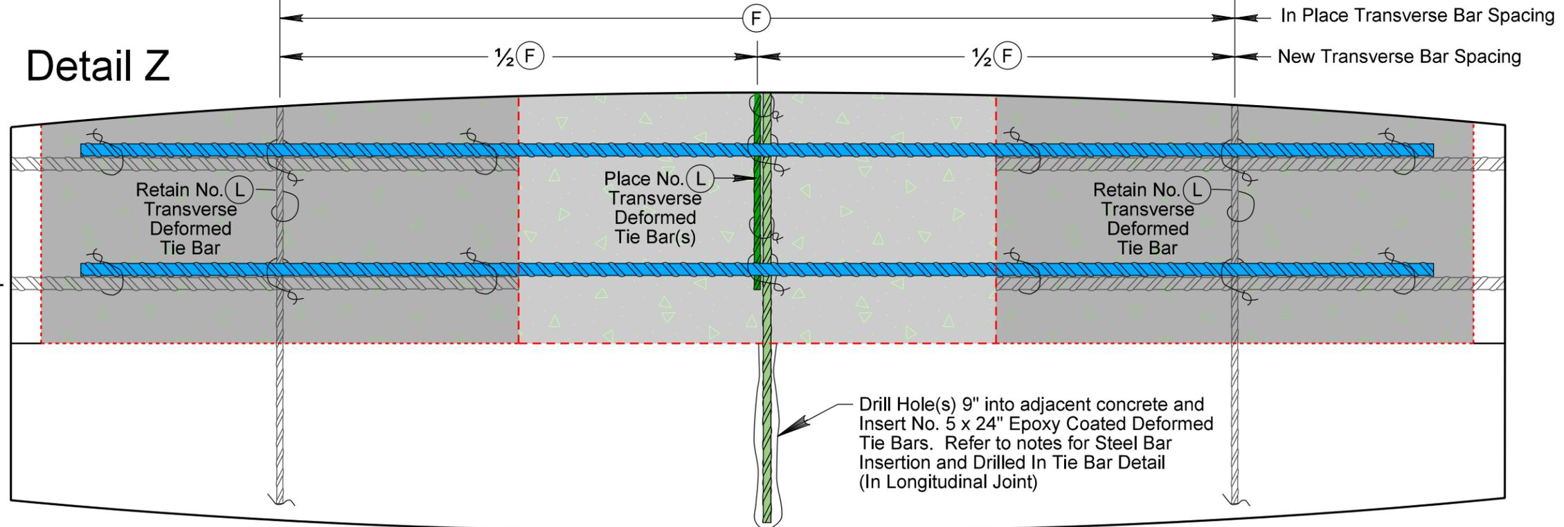
For Repair Area Length L = 8' or more - every other in place No. (C) Longitudinal Deformed Tie Bar shall be cut off and lap splices shall be staggered similarly to the details for CRC PAVEMENT REPAIR AREA (FULL LANE WIDTH).
