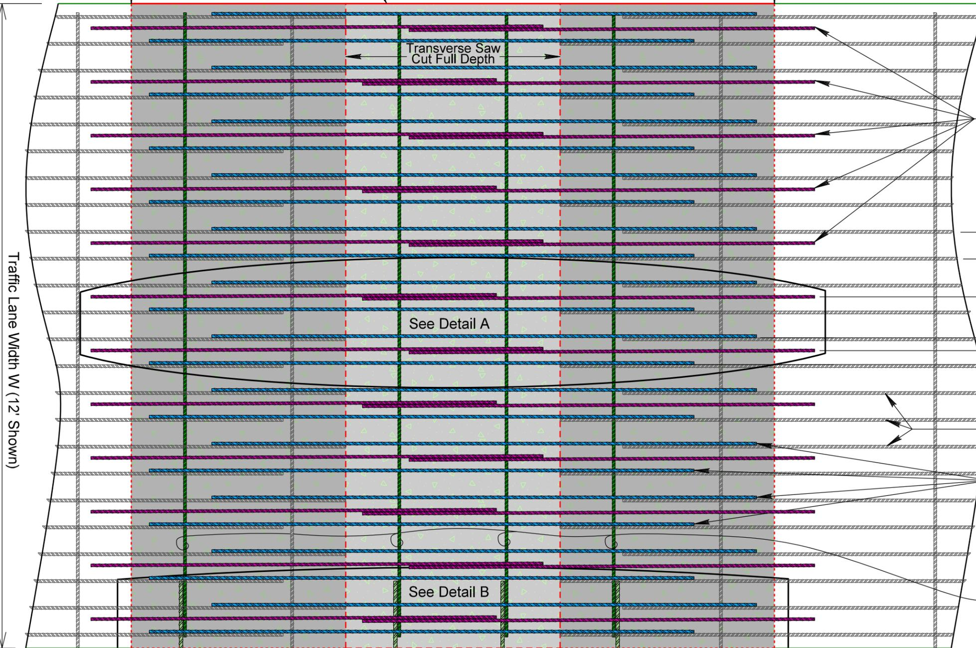
Place No. (C) Longitudinal Deformed Tie Bar (Place bars into drilled holes in existing concrete on both sides of the repair area and tie the bars to each other and to in place No. (L) Transverse Bars)
