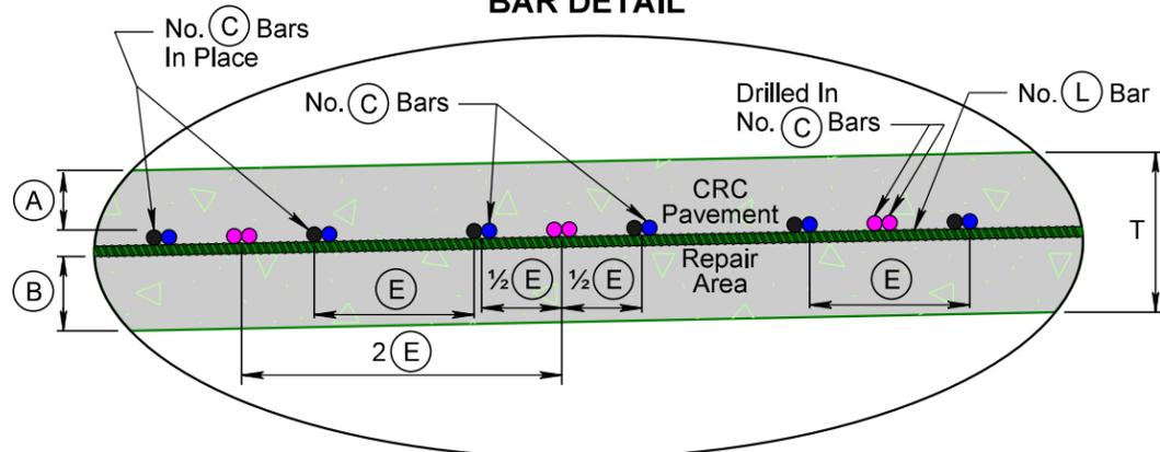
Placement of longitudinal steel bars may vary from +1/2" to -1/2" vertically and 3/4" horizontally. Placement of transverse steel bars may vary from +1/2" to -1/2" vertically and 2" horizontally.
