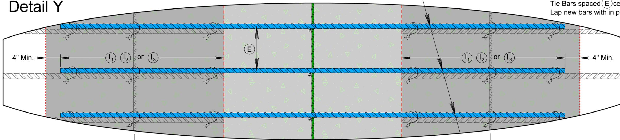
Place No. (C) Longitudinal Deformed Tie Bars spaced (E) center to center. Lap new bars with in place bars.
