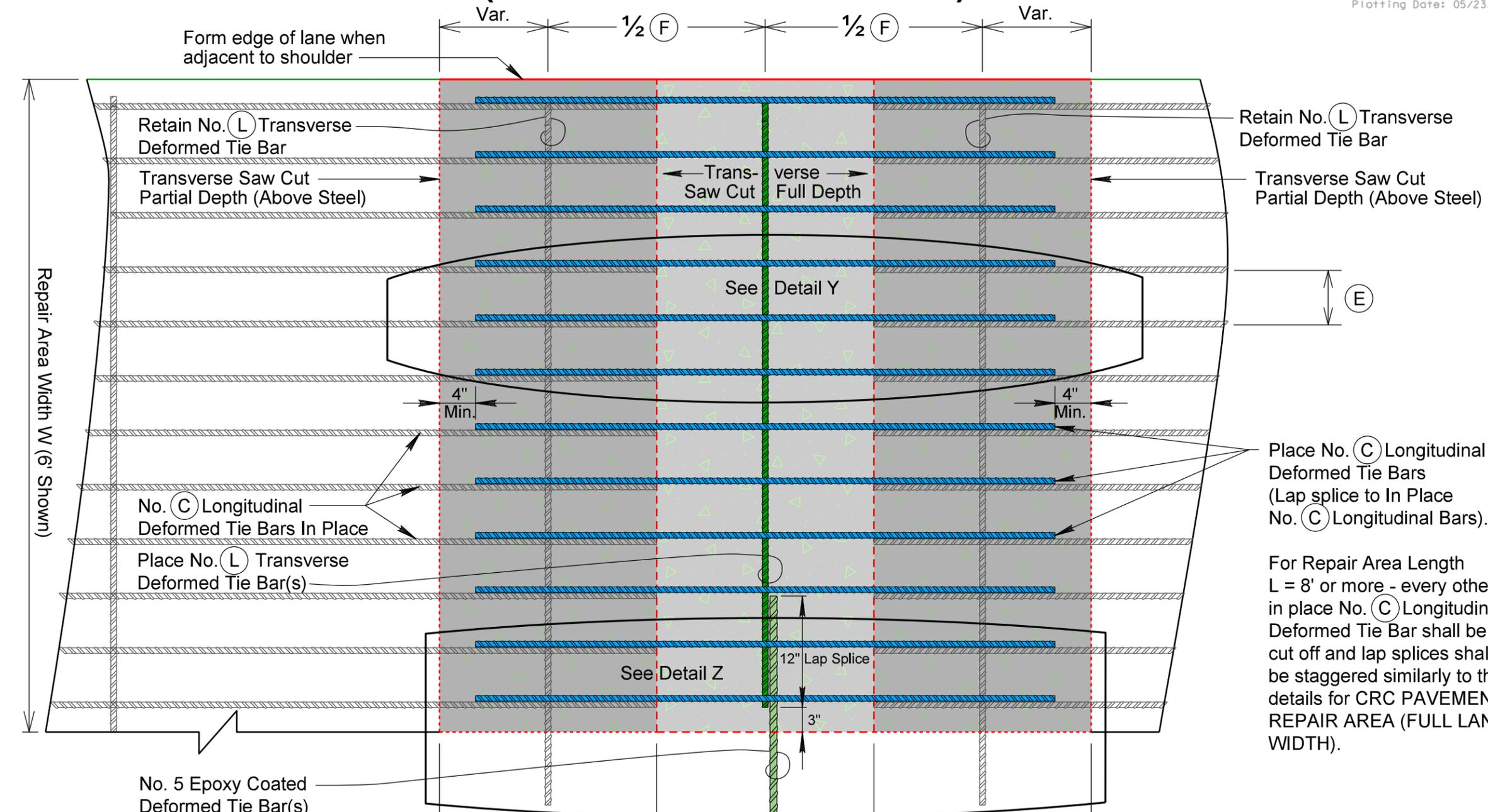
Place No. (C) Longitudinal Deformed Tie Bars (Lap splice to In Place No. (C) Longitudinal Bars).
