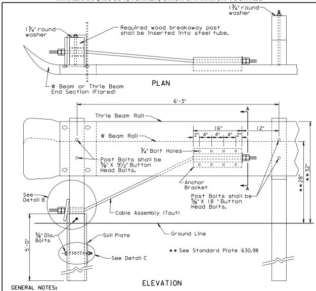
All hardware shall be galvanized in accordance with ASTM AI53.
