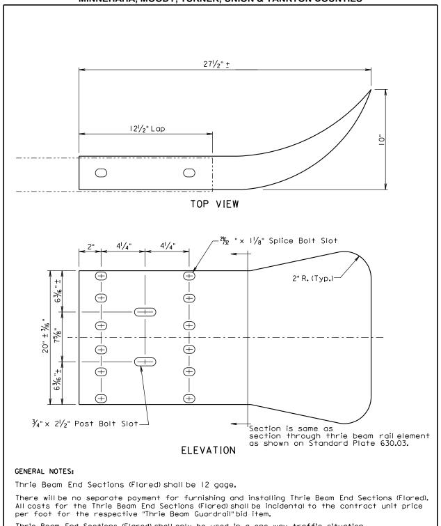
Thrie Beam End Sections (Flared) shall only be used in a one way traffic situation. See Standard Plate 630.80 for Thrie Beam End Section (Flared) in the Beam Guardrail Trailing End Terminal.
