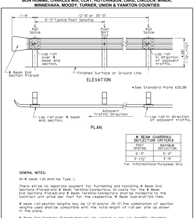
W Beam End Sections (Flared) shall only be used in a one way traffic situation. See Standard Plate 630.80 for W Beam End Section (Flared) in the Beam Guardrail Trailing End Terminal.
