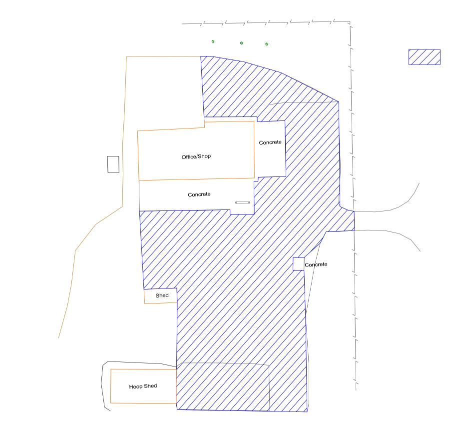
Two - 2" Asphalt Concrete Composite Lifts 60,444 SqFt - 6716 SqYd 1490 Tons Asphalt Concrete
