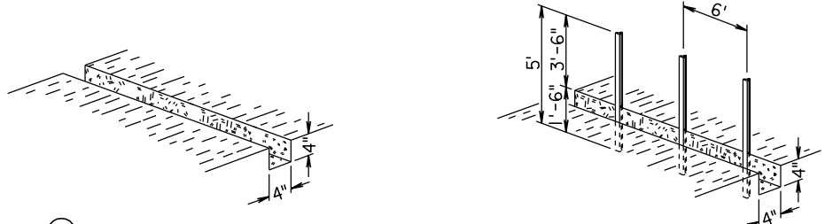
① EXCAVATE TRENCH
