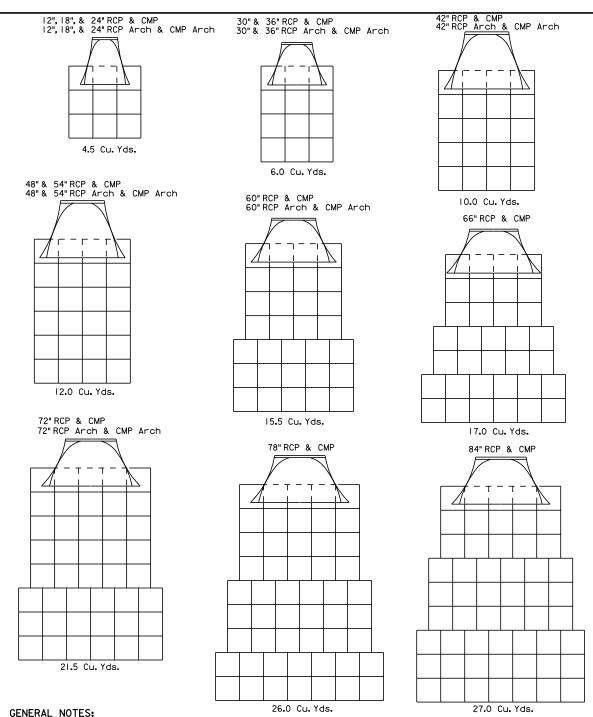
Gabions at outlets of C.M. pipe and R.C. pipe shall be placed under the end section a distance of 2' from the outlet end of the section. For C.M. pipe end section installations, the upper fabric of the gabions shall be modified to accommodate the metal end section in a manner approved by the Engineer.
