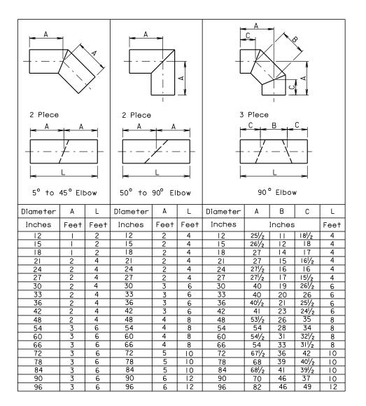
FABRICATED ELBOW LENGTHS FOR ALL CORRUGATIONS
