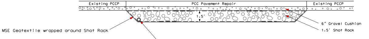
Install 20' of 4" Corrugated Polyethylene Drainage Tubing to drain water from the shot rock. The tubing shall be placed at the lowest point and shall outlet through the inslope.
