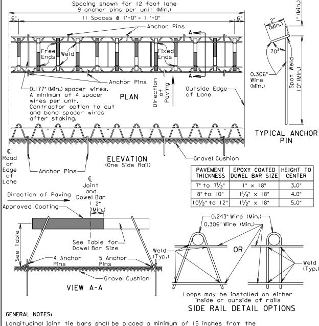
Longitudinal joint tie bars shall be placed a minimum of  ${\sf I5}$  inches from the transverse contraction joint.
