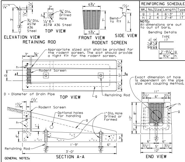
The concrete shall be Class M6. The concrete shall conform to the requirements of section 462 of the Standard Specifications. It is estimated that each unit weighs approximately 210 pounds.
