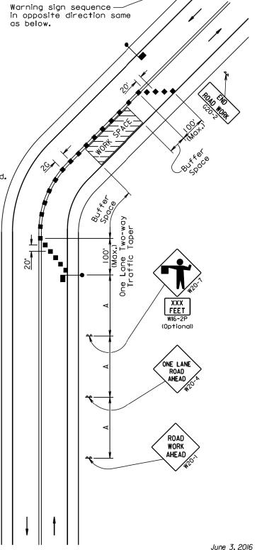
**GUIDES FOR TRAFFIC CONTROL DEVICES** LANE CLOSURE WITH FLAGGER PROVIDED PLATE NUMBER 634.23
