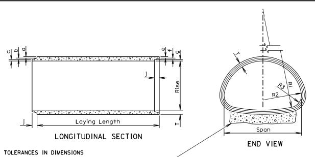
Radial dimensions at joints:  $\pm \frac{1}{8}$ " for 65" span or less and  $\pm \frac{1}{4}$  for longer spans. Rise and Span: +2% of tabular values. Length of Joint (J):  $\pm \frac{1}{4}$ ". Wall thickness (T): not less than design T by more than 5% or  $\frac{3}{6}$ ", whichever is greater.
