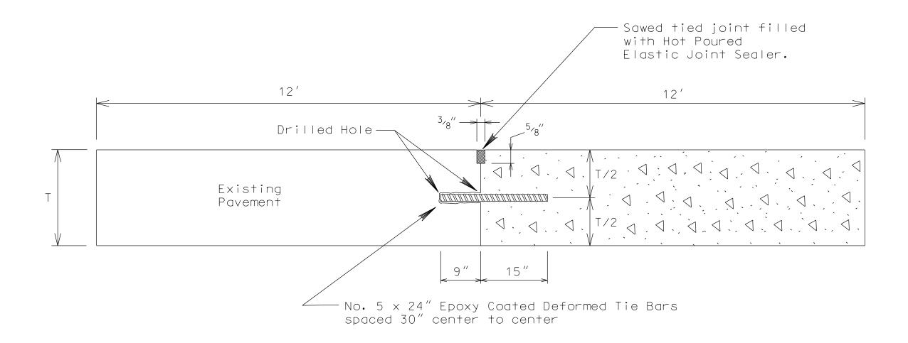
T = New existing and new pavement thickness.
