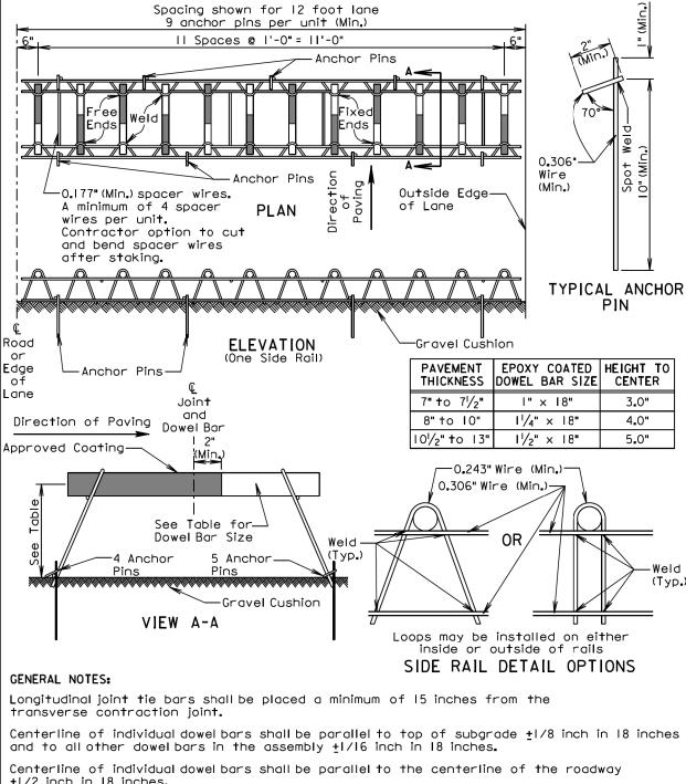
Centerline of individual dowel bars shall be parallel to top of subgrade ±1/8 inch in 18 inches
