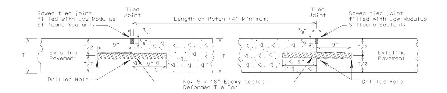
T = Existing and new pavement thickness.
