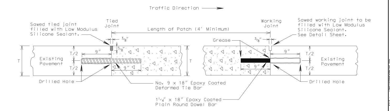
T = Existing and new pavement thickness.
