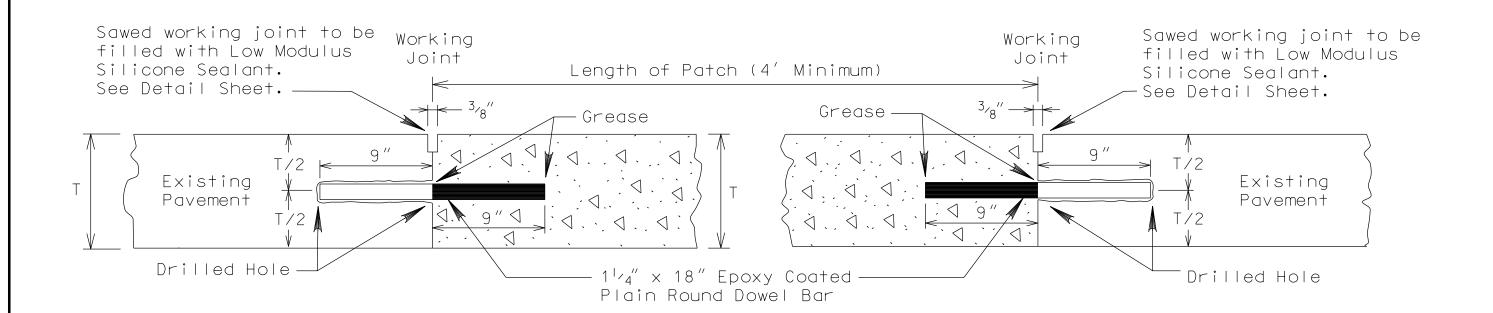
T = Existing and new pavement thickness.
