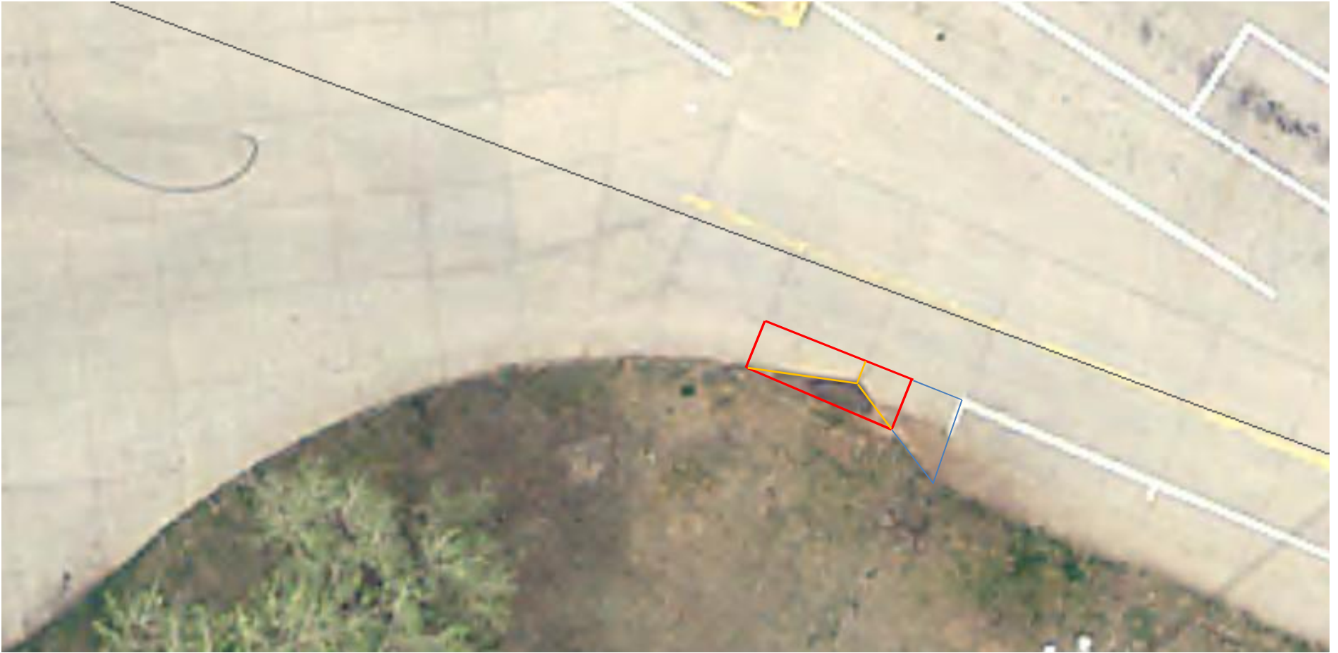
Wasta Eastbound truck turn-around: remove 108.5 sq ft, place 155.8 sq ft (23'-8" by 79")
