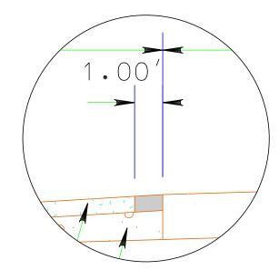
Remove and Place 3" Asphalt Concrete Composite Adjacent to PCCP.
