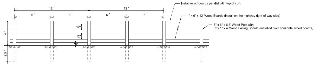
\* Over uneven ground the 6" clearance will vary. In low areas backfill and tamp around posts to meet the 2.5' post embedment depth.
