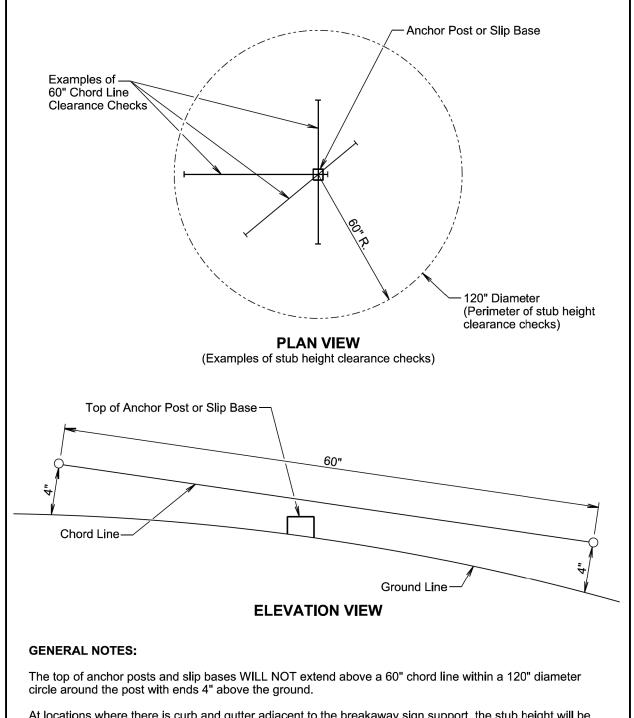
At locations where there is curb and gutter adjacent to the breakaway sign support, the stub height will be a maximum of 4" above the ground line at the localized area adjacent to the breakaway support stub.
