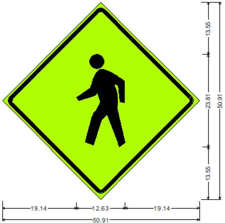
36.00" across sides 0.88" Border, 0.63" Indent, Black on Yellow Green; Pedestrian Symbol White;
